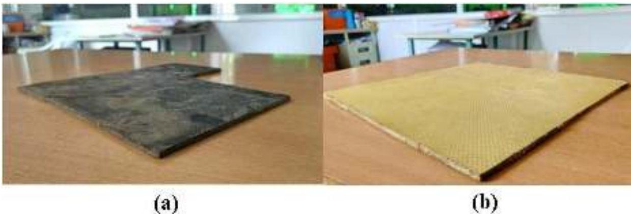
Fabricated Hybrid Laminate: a) Kevlar/E-Glass Laminate; b) Basalt/E-Glass Laminate
