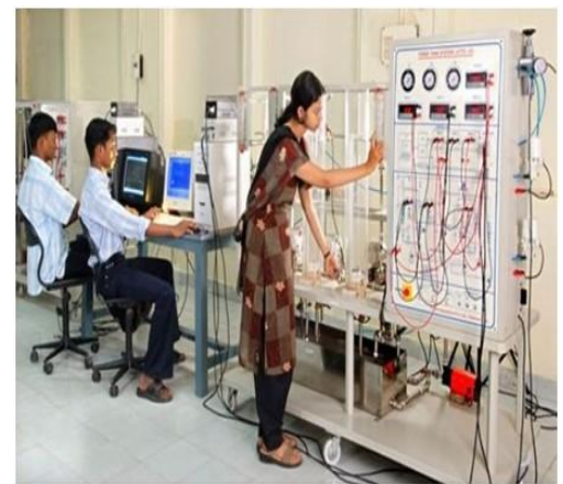
School of Electrical & Communication Sciences Three Tank interacting cylindrical Level Process with Closed loop Control Setup
