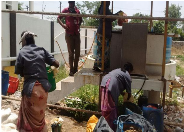
Food waste feed in to Bio gas plant
