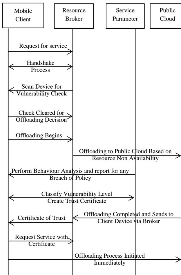
Figure. 4 Sequence depiction of Trusted Mobile-Cloud Environment
